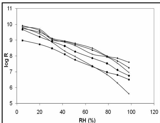
**Fig. 2** RH vs  $\log R$  plot of NiWO<sub>4</sub>–WO<sub>3</sub> composites
