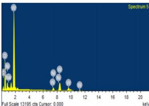
**Fig. 1a** EDAX spectrum for synthesized NiWO<sub>4</sub> – WO<sub>3</sub>
