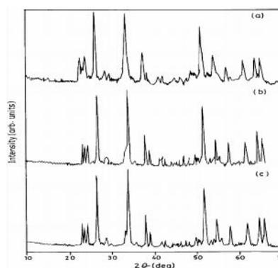
**Fig. 1b** Powder XRD of NiWO<sub>4</sub> – WO<sub>3</sub> composites (a) NWWO-64, (b) NWWO-46 and (c) NWWO-28
