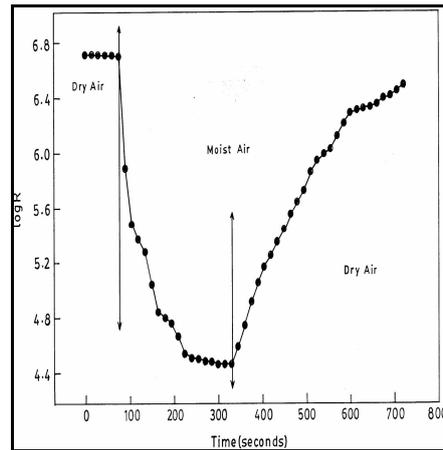
**Fig. 4** Response and recovery behaviour of NWWO-46 composite.
